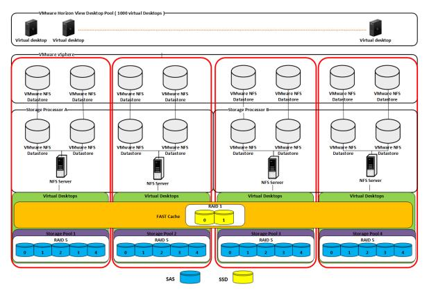
Figure 3. Storage building block for desktops
