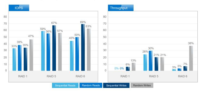
Figure 1. Front-end I/O performance improvement of vSAN 7.0 U1 over 7.0
