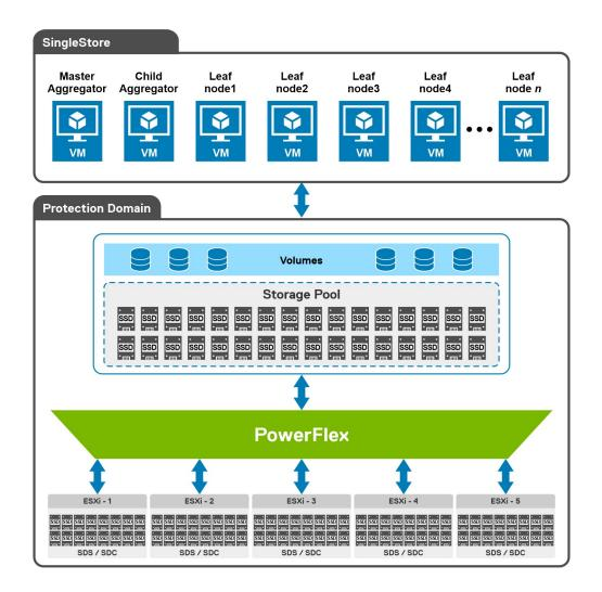
For this validation, the SingleStore Cluster VMs consist of two aggregator VMs and multiple leaf VMs. The white paper details the configuration of these VMs.
